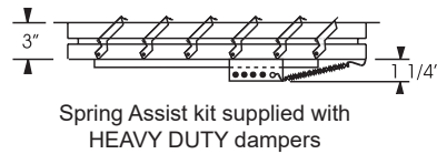
DETAIL #2 Two panel damper for ventilator size 42 & larger.
