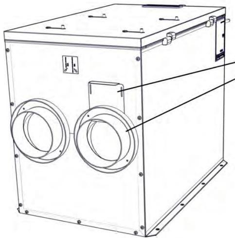
Fit damper between duct collar and unit for the stream with the higher airflow.
