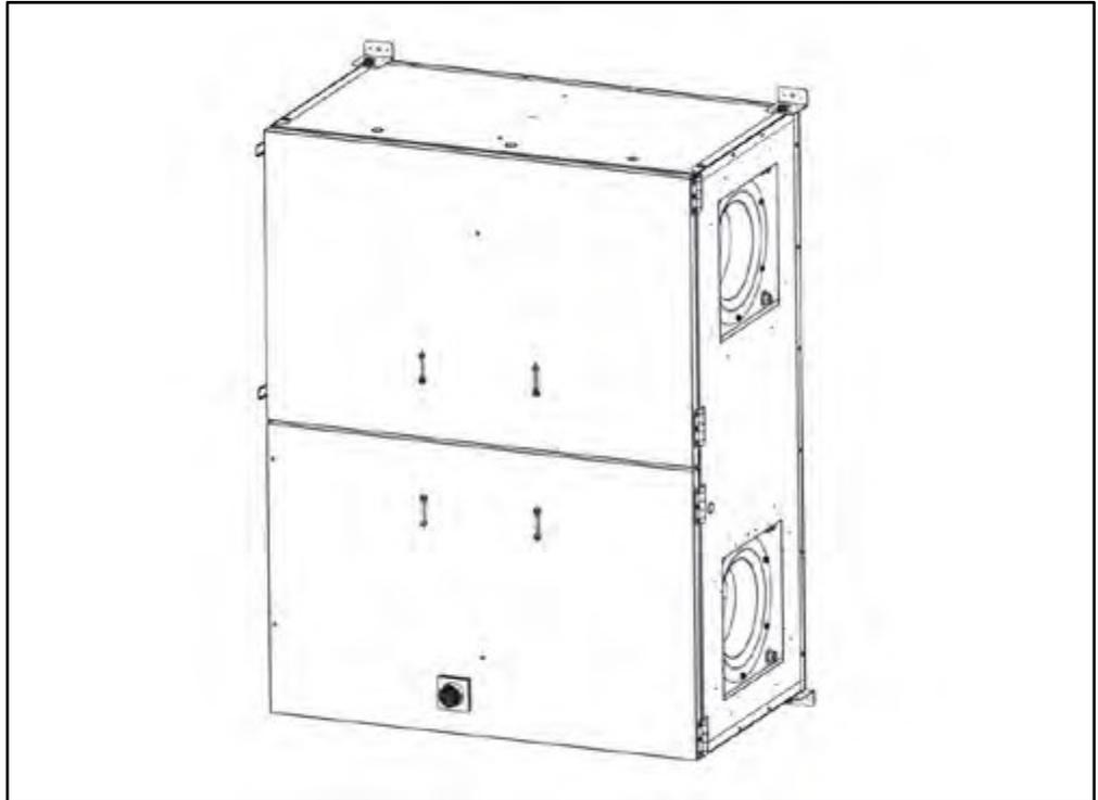
FIGURE 5.3.1 KIT DE SUPPORT DE SUSPENSION
