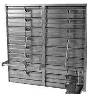
The flanged frame damper is designed to recess inside the flanges of the optional wall housing or wall mounting collar. The center pivot style damper provides superior weather resistance. Galvanized (optional aluminum) construction is rated to 3500 FPM with proper clearance as provided by all factory accessories.
