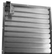
The motorized option improves weather protection by providing a tighter closure seal and is recommended for all supply applications. Standard duty dampers are constructed with galvanized frames and aluminum blades and are rated to 2000 FPM. The damper body is not recessed providing extra clearance between the fan and damper blades.
